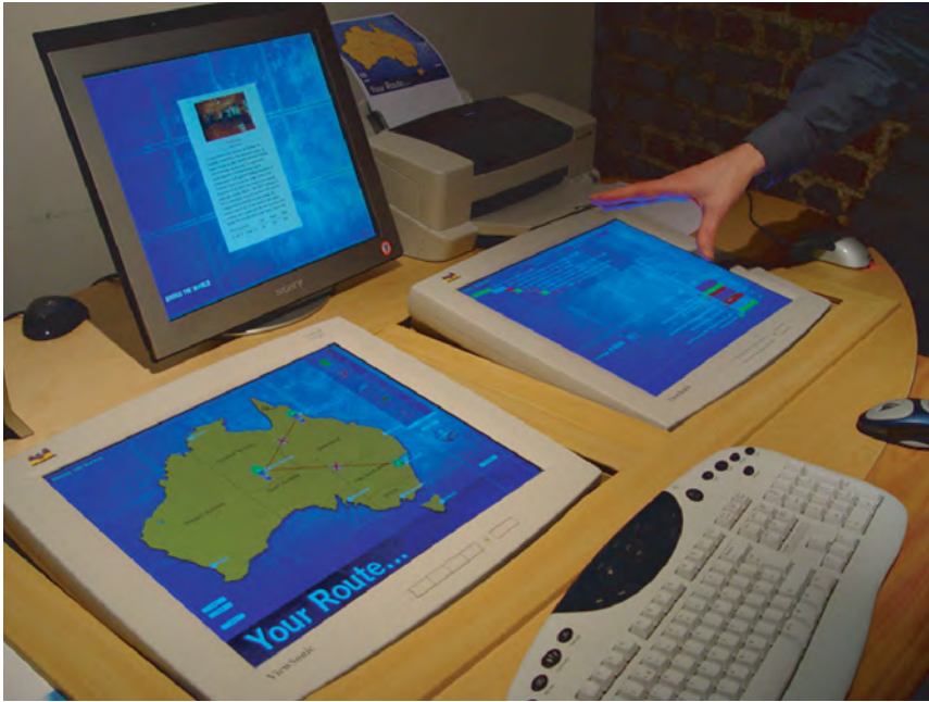
Figure 11 The second version of the eTable with three interlinked displays using wireless keyboard and mouse for input
