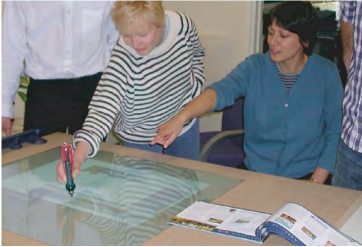
Figure 10 The first version of the eTable using horizontal shared screen and Mimio pen for input
